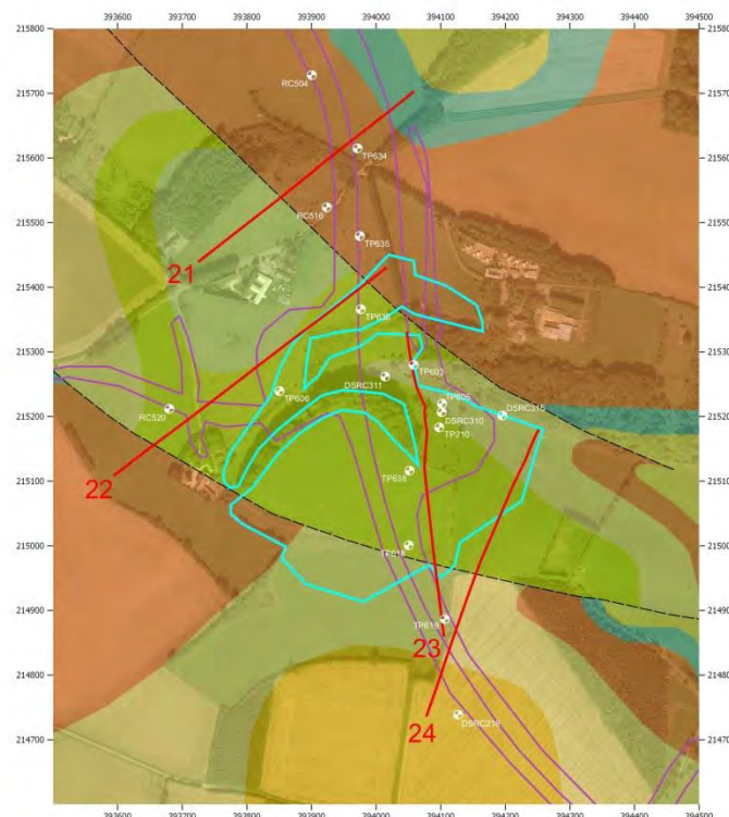
Plate 1. Zone 3, showing the locations of the ERT and seismic profiles (red lines) and the extents of the EM ground conductivity survey (light blue).
