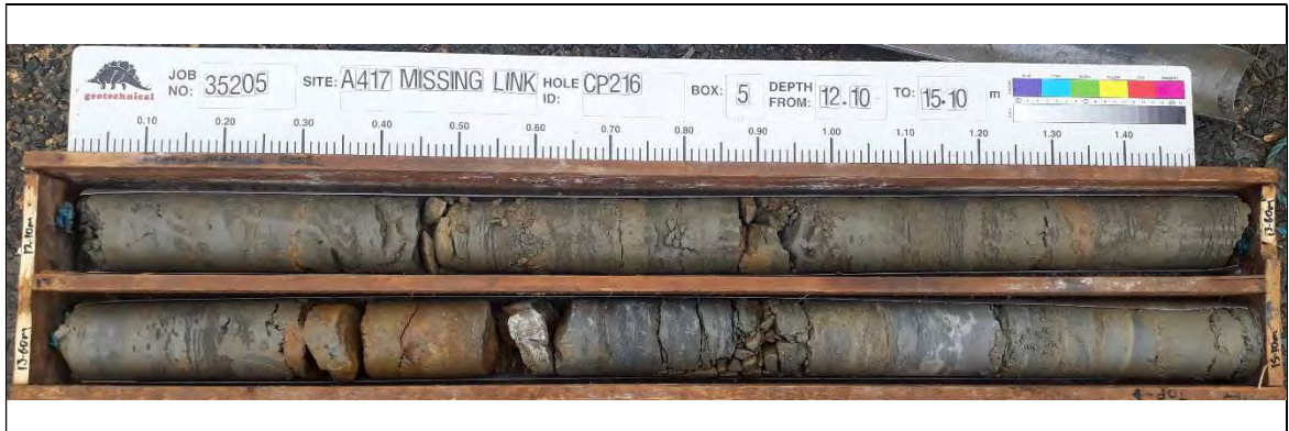
Borehole: CP216 Box 5 12.10-15.10m
