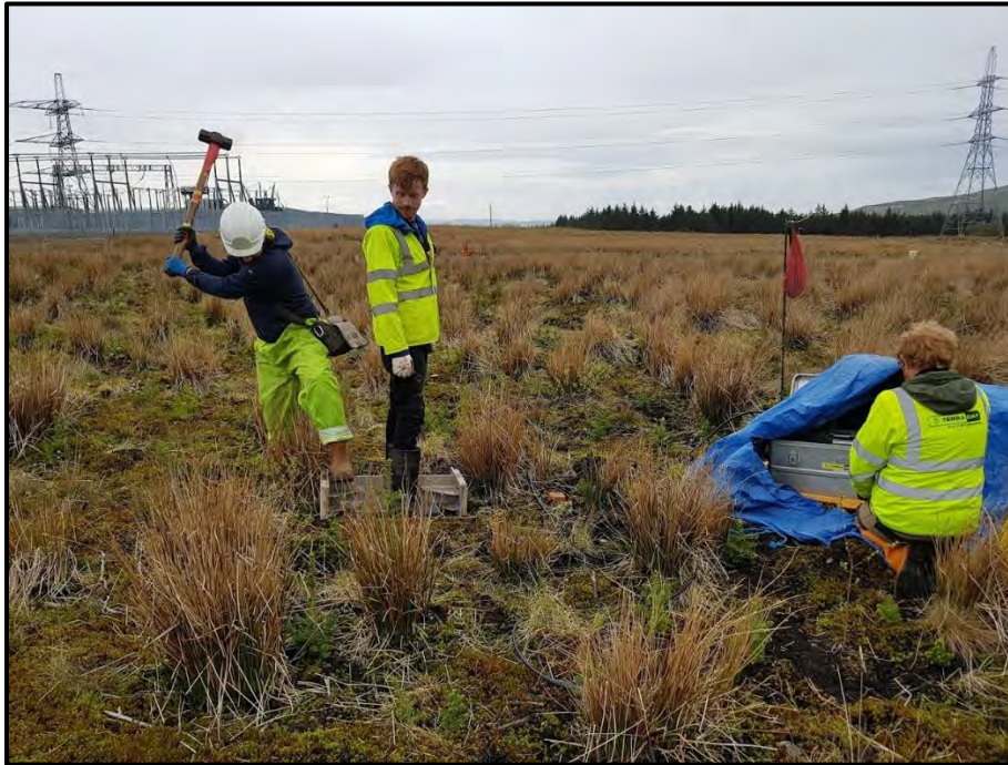
Plate 5. S-wave source plate being struck (Library photo).
