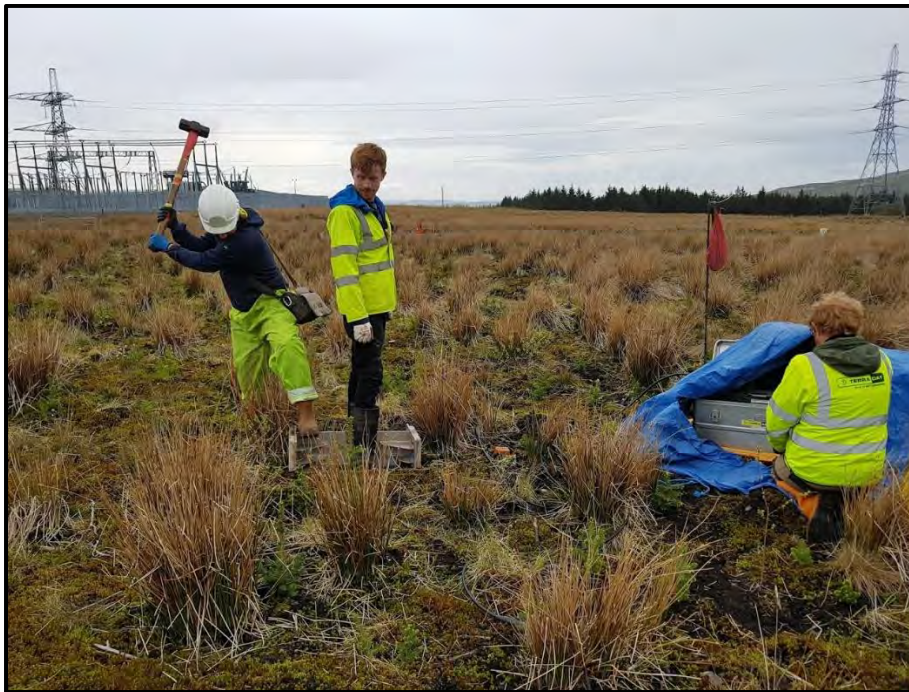
Plate 4. S-wave source plate being struck (Library photo).
