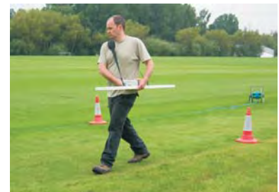
GEM-2 Multi-frequency Exploration depth up to 10m
