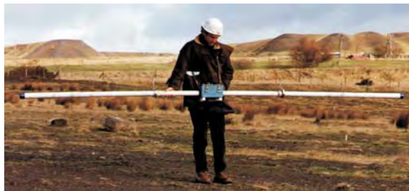
EM-31 Single frequency Exploration depth ~3 to 5m
