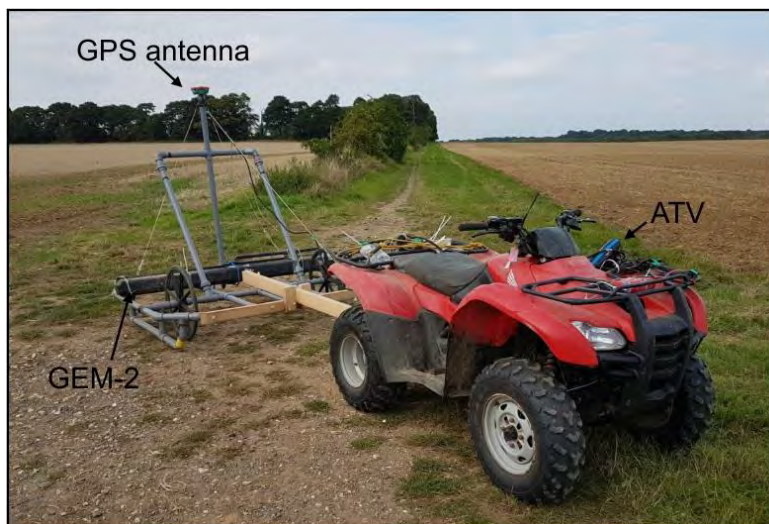
Plate 2. Ground conductivity data collection method. Geophex GEM-2 instrument mounted on a bespoke cart which was pulled across the site using an ATV, under the control of a GPS system (Library photo).
