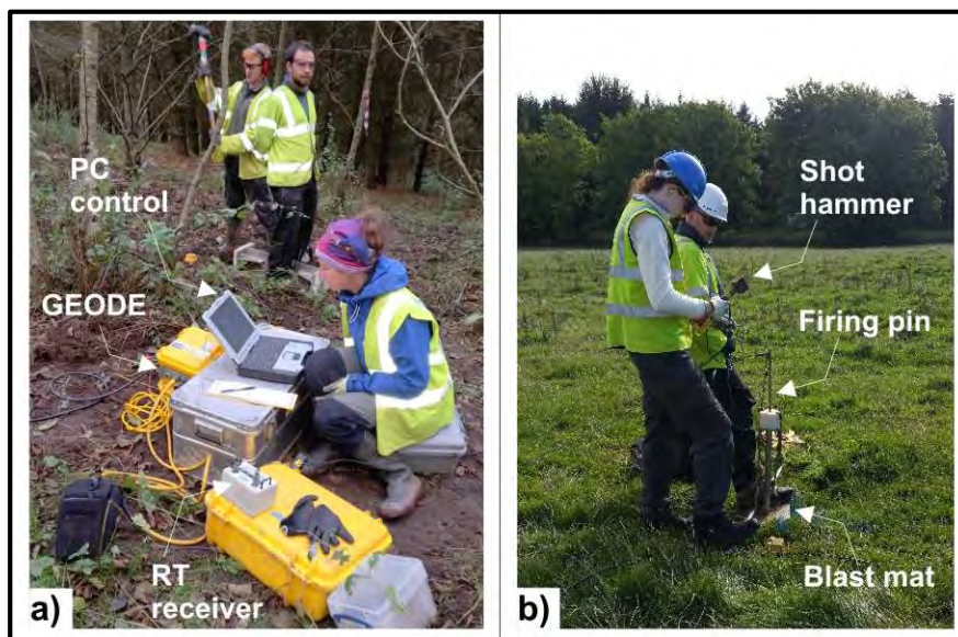
Plate 4: a) Field set-up and b) Seismic Impulse Source deployment (library picture).
