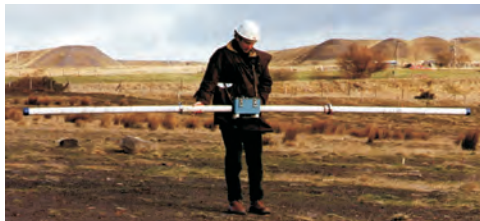
EM-31 (Exploration depth ~3 to 5m)
