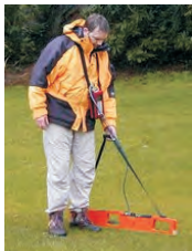
EM-38 (Exploration depth ~1.5m)
