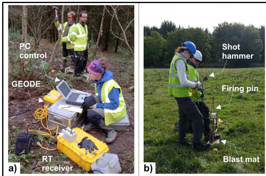
Plate 3. a) Field setup and b) Seismic Impulse Source deployment (Library picture).
