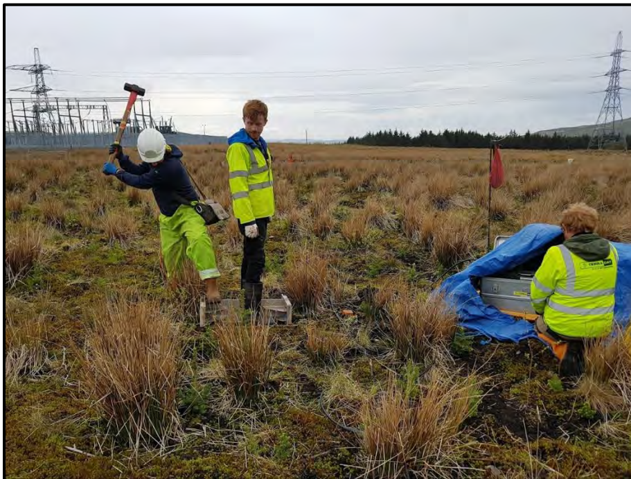
Plate 5. S-wave source plate being struck (library photo).
