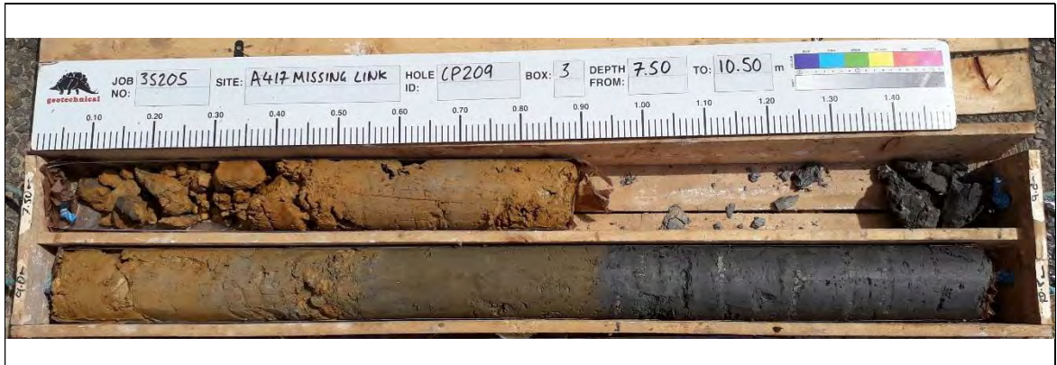
Borehole: CP209 Box 3 7.50-10.50m
