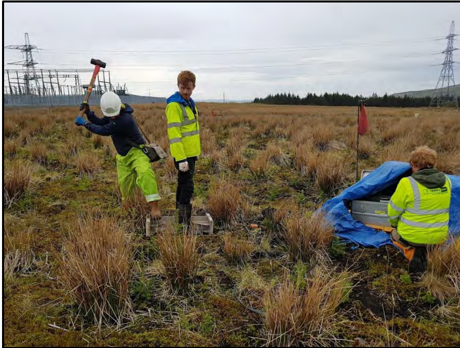
Plate 5. S-wave source plate being struck (Library photo).
