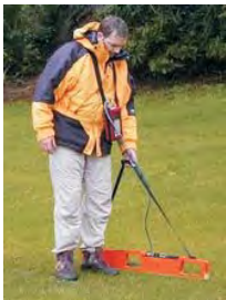
EM-38 Single frequency Exploration depth ~1.5m
