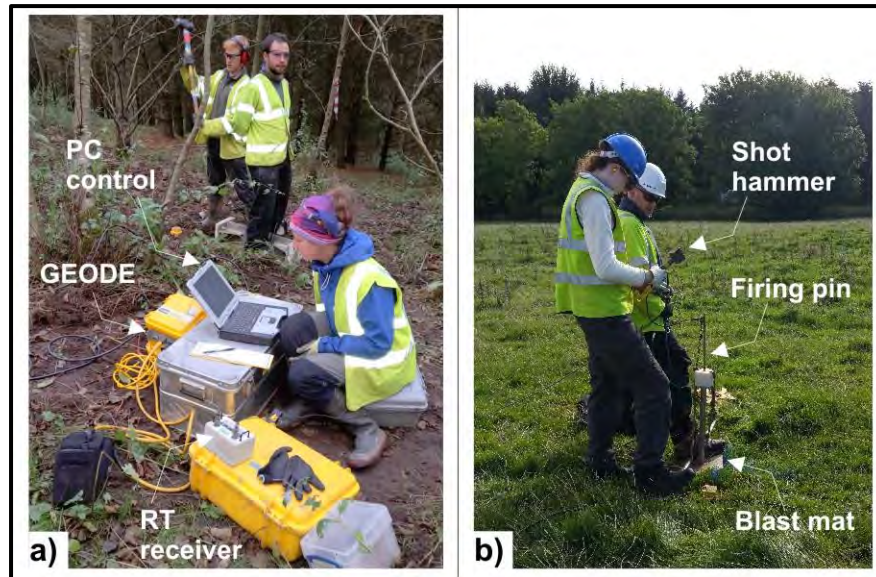
Plate 4. a) Field setup and b) Seismic Impulse Source deployment (Library photo).
