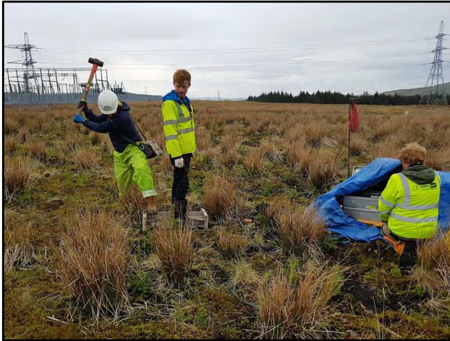
Plate 5: S-wave source plate being struck (library photo)
